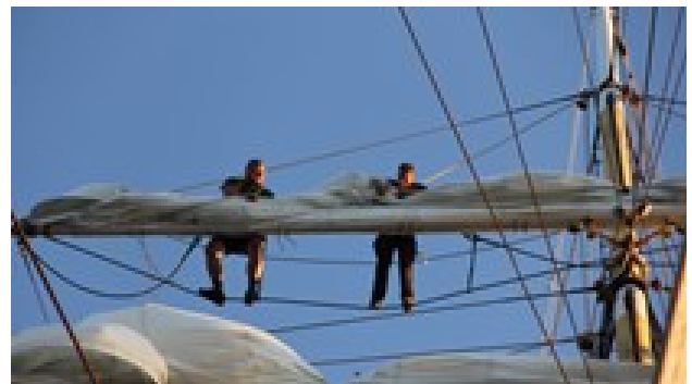
Scatchard, John, 2014, Two men at the yards, standing on a footrope and setting the sail on the Statsraad Lehmkuhl ( https://lehmkuhl.no/en/ )
