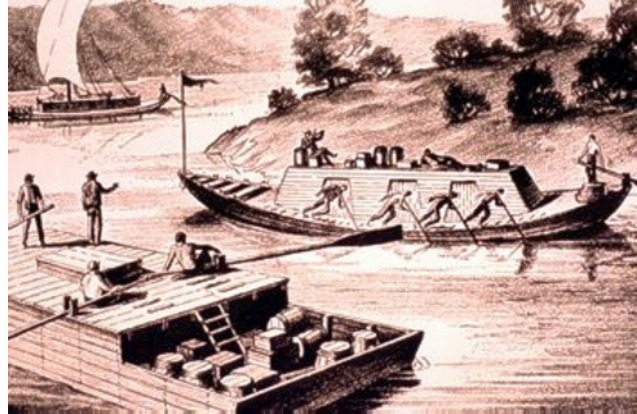
Flatboat (foreground) and Keelboat, around Pittsburgh, late 18th century. via wikimedia commons
